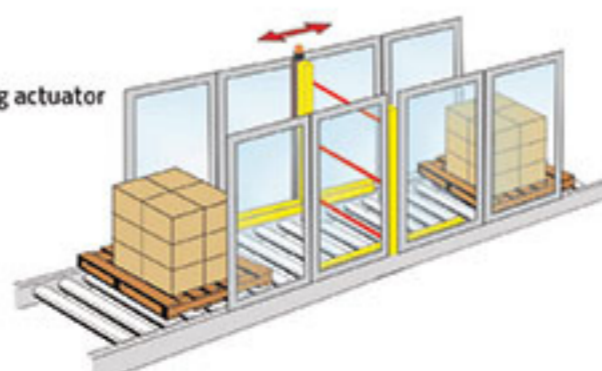
Fig. 8 Safety Light Curtain with Integrated T muting actuator
